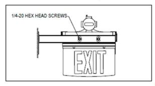
Attach conduit to hub on the fixture, making sure that at least five full threads are engaged and conduit is tight as per the requirements of the NEC.
