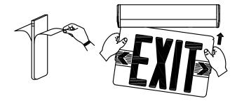
7. Determine direction for chevron placement. (See DETERMINE DIRECTION)
