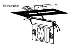
7. Insert fixture into metal box and snap by spring, fix trim plate on the metal box by 2 screws.
