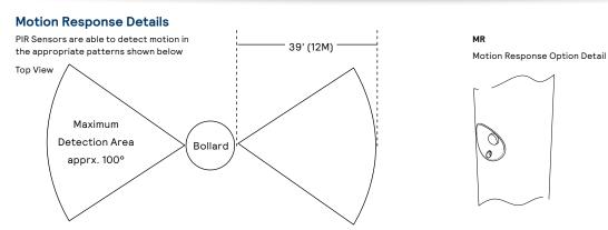
Note: Motion Sensors rely on special zonal crossings to detect motion. It is possible for a person to directly approach the bollard motion sensor without crossing between zones until 15' from the motion sensor. The actual motion detection distance may vary based on specific application characteristics.
