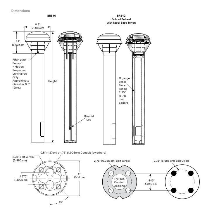
**NOTE**: Factory supplied template must be used when setting anchor bolts. Gardco will not honor any claim for incorrect anchorage placement from failure to use factory supplied templates.
