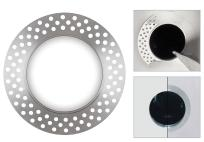
Mud-in ring (FT): Low profile, machined aluminum mud-in ring provides a raised rib to plaster up to and a 3/16" flange thickness. The ring is attached to the ceiling material as opposed to the frame-in kit to avoid conduction of heat and vibration which can cause yellowing or cracking of the plaster.
