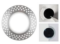
Mud-in ring (FT): Low profile, machined aluminum mud-in ring provides a raised rib to plaster up to and a 3/16" flange thickness. The ring is attached to the ceiling material as opposed to the frame-in kit to avoid conduction of heat and vibration which can cause yellowing or cracking of the plaster.
