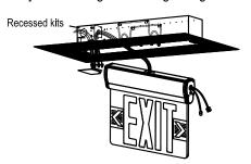
8. Insert fixture into metal box and snap by spring, connect test switch, assemble LED indicator on bushing at trim plate. fix trim plate on the metal box by 2 screws.
