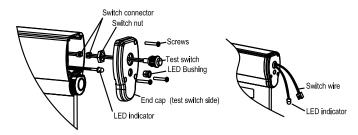
3. Unscrew and remove trim plate from metal box, fix test switch and LED bushing on the trim plate.
