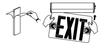
7. Determine direction for chevron placement. (See DETERMINE DIRECTION)
