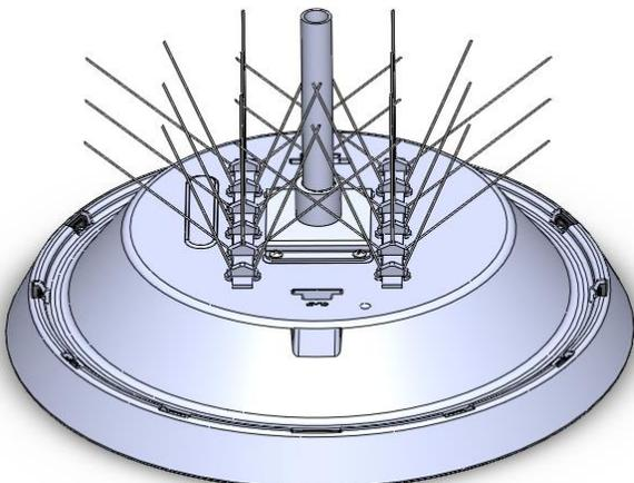
Spike bird deterrent option is primarily used for pendant application. Additional trimming of the strip may be required. Bending the individual pins may be required for coverage of flat areas where birds might want to nest.
