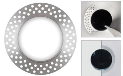
**Mud-in ring (FMR):** Low profile, non-metallic mud-in ring provides a raised rib to plaster up to and a 3/16" flange thickness. The ring is attached to the ceiling material as opposed to the frame-in kit to avoid conduction of heat and vibration which can cause yellowing or cracking of the plaster.
