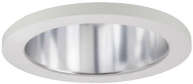
**Vandal proof (VP):** Provides an elegant solution for vandal resistant needs. One piece machined aluminum ring with impact resistant clear lens. Flangeless (F) flange must be ordered. Provides the luminaire with an IK10 impact and IP65 rating.
